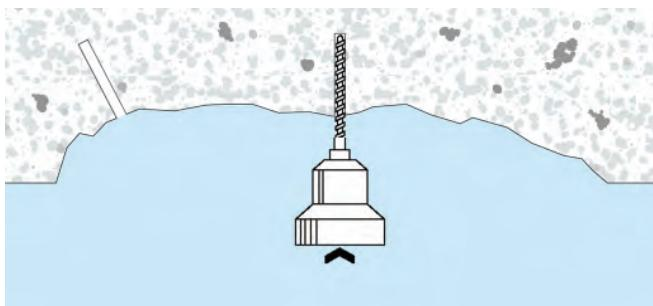
2. Drill pilot holes, vertically or at an angle of up to 45°, to the correct diameter and spacing into the concrete (using an SDS rotary hammer drill).
