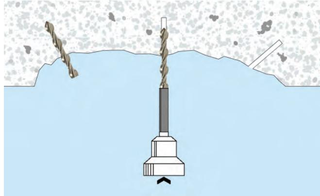
3. Fit the PatchPin support tool over the drill bit and insert the PatchPin into the tool. Install the PatchPin into the pilot hole with the SDS rotary hammer drill set to hammer only. Ensure that the outer end of the pin will be below the face of the concrete patch – the pin can be bent, if required.
