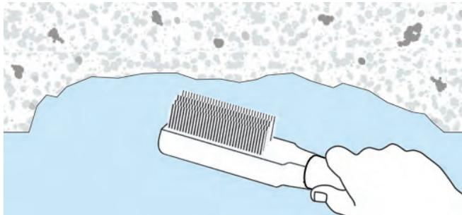
1. Remove all loose concrete from the area to be patched. Hammer tap the area to establish if any hollows are present and break back to sound concrete. Remove any dust and debris with a stiff wire brush. Clean and treat any exposed embedded steel rebar with a suitable epoxy coating.
