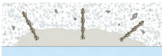
4. Apply the patching mortar, as required, in accordance with the Manufacturer's instructions. Fill all gaps and make good the surface.
